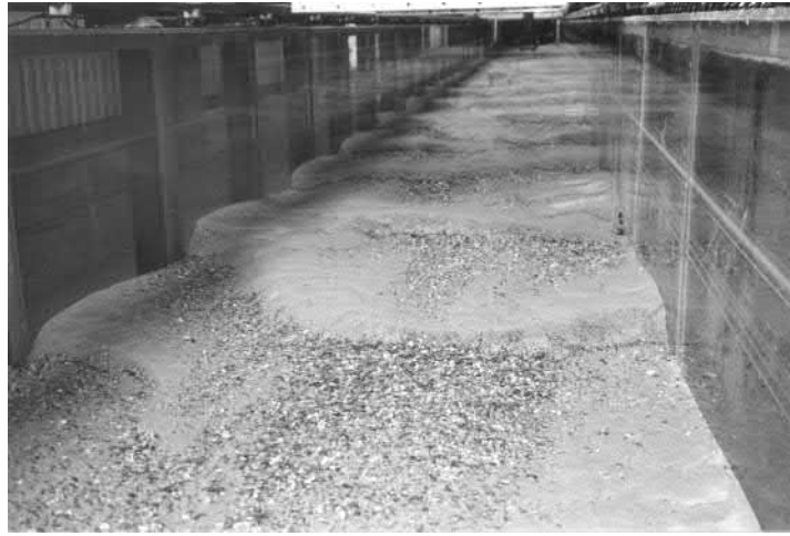
Figure 3.1 Bed form pattern from T7 experiment at equilibrium conditions (from (Blom et al. , 2003))
