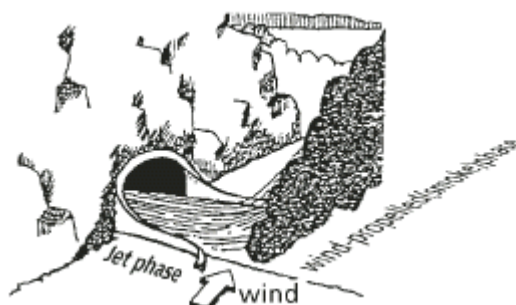
Figure A.1 Jet phase and smoke phase
