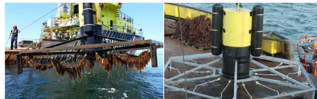
First seaweed production system used by North Sea Farmers in 2015. It is a wheel-based system with a diameter of five metres. The seaweed was grown at a depth of about two metres.
