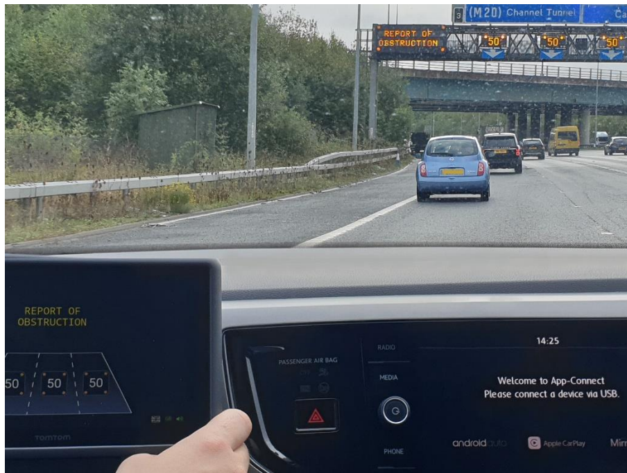
Figure 70: UK HMI installed in vehicle displaying IVI on the M2 in Kent during a UK TESTFEST
