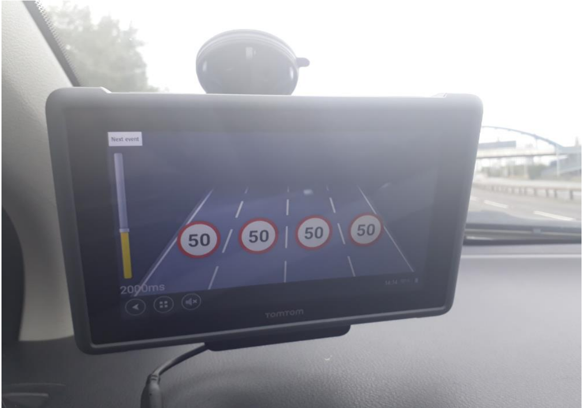
Figure 69: UK supplied HMI displaying IVI messages on the A102 in London
