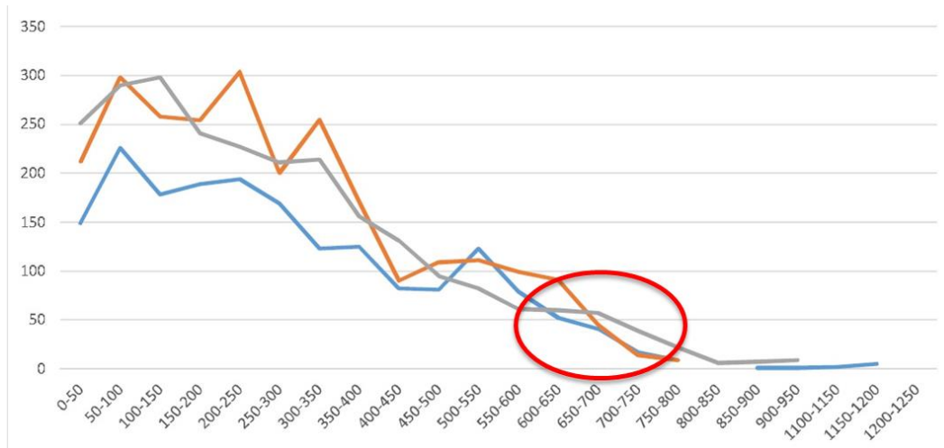
Figure 23: Number of messages received as a function of the distance to the trailer (results from three different vehicles)
