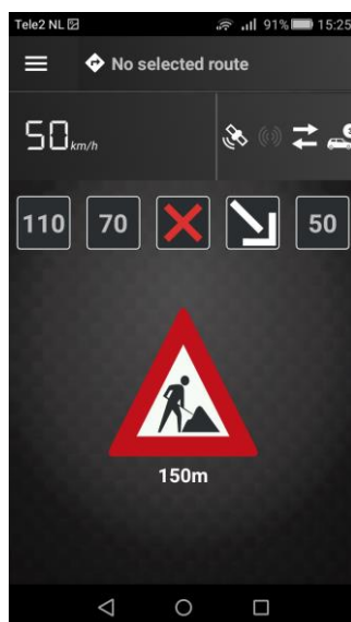
Figure 12: HMI of the application using the ITS-G5 channel + OBU
