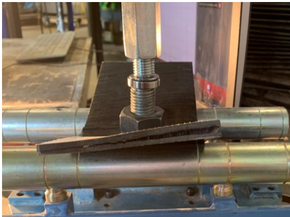
Figure 6-1 Fail with crack to right edge (1)
