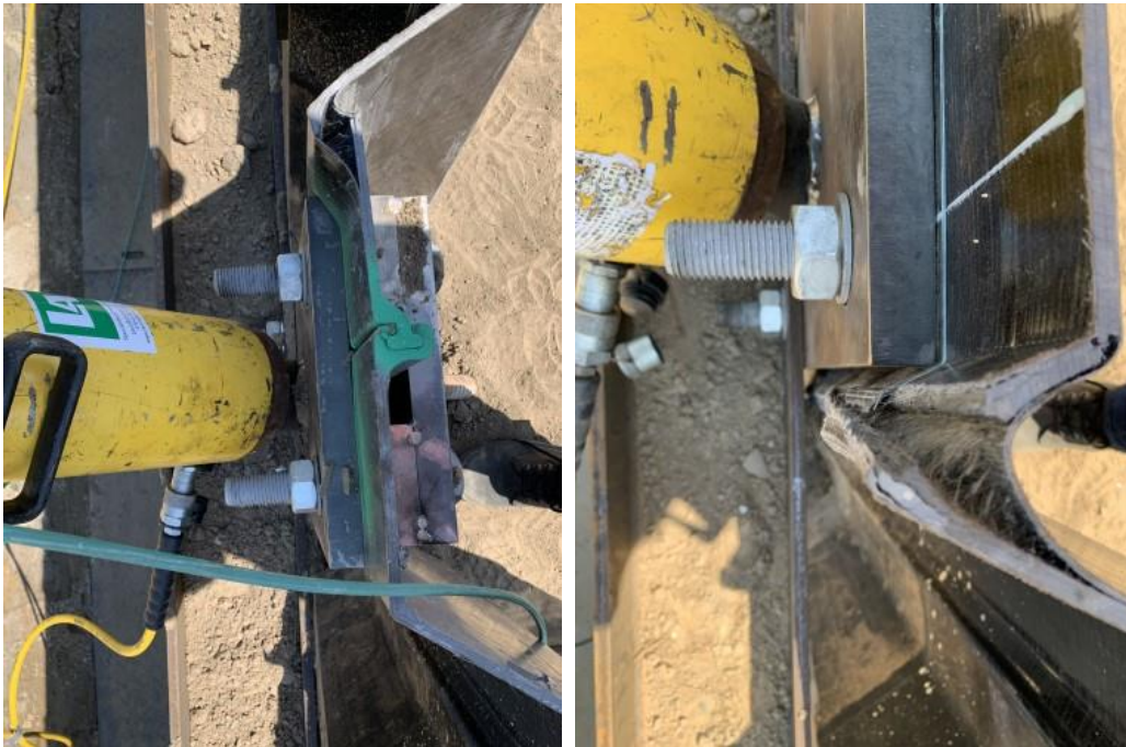
Figure 9-13 Local buckling and delamination of the outer 0/90 laminate layer
