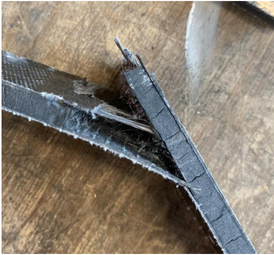
Figure 6-2 Failure mechanism transverse (2)
