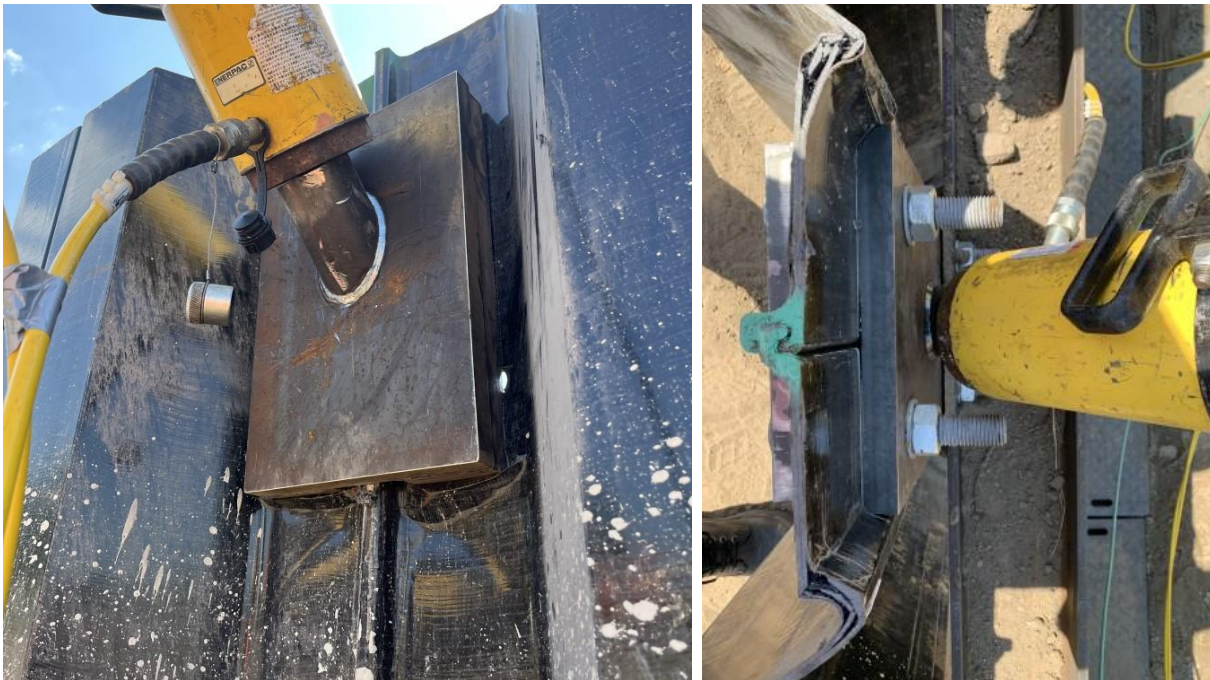
Figure 9-12 Local buckling and delamination of the outer 0/90 laminate layer
