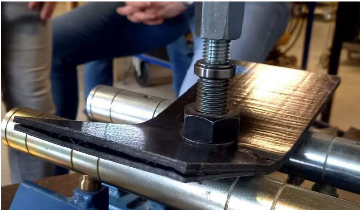
Figure 4-6 Complete failure (interlaminar shear)
