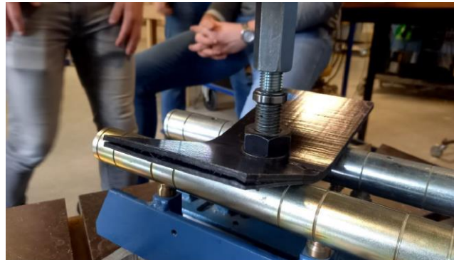
Figure 6-2 Fail with crack to right edge (2)
