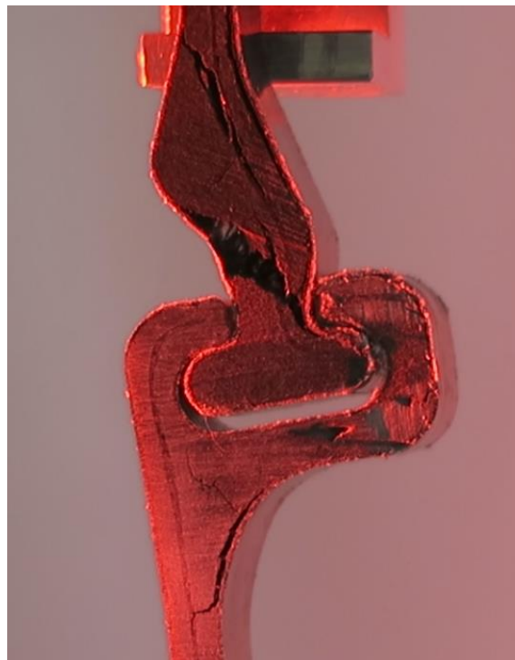
Figure 6-4 Final failure mechanism (1)
