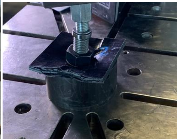
Figure 6-4 Bad delamination due to support cylinder (2)
