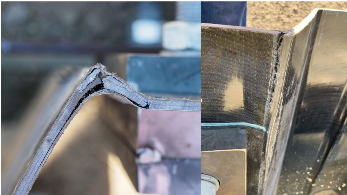
Figure 9-10 delamination and failure of the outer laminate layer
