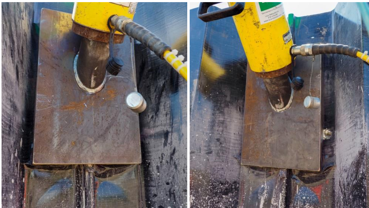
Figure 9-8 Local buckling and delamination of the outer 0/90 laminate layer
