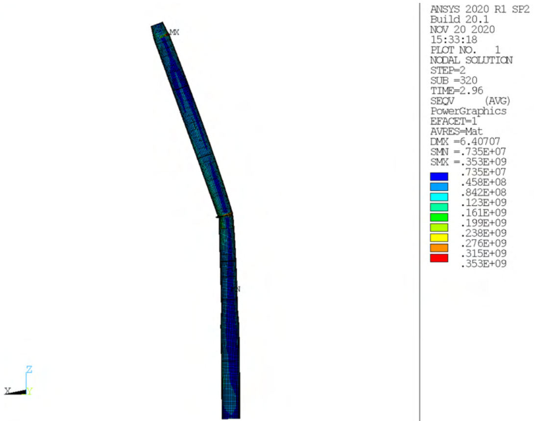
Figure A 23: Chemical tanker , end deformation and Von Mises stress in [Pa], Drifting.
