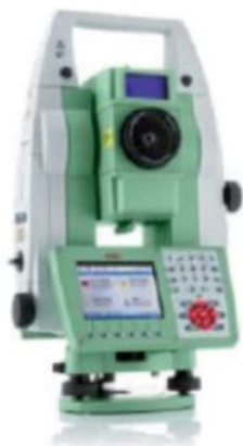
Figuur 5.6 / Robotic total station, RTS.
