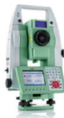
Figuur 5.6 / Robotic total station, RTS.
