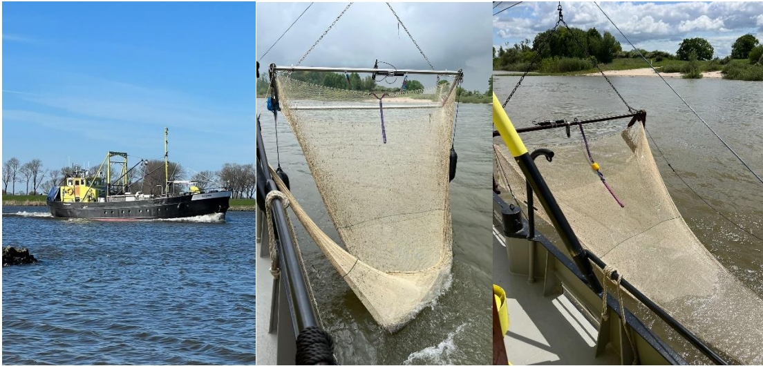
Figure 9 - From left to right: The Stern, the ship from which the samples were taken. The trawl (4x1m) hanging on the side of the ship, both on port and starboard. The trawl being lowered into the water to collect plastic samples.
