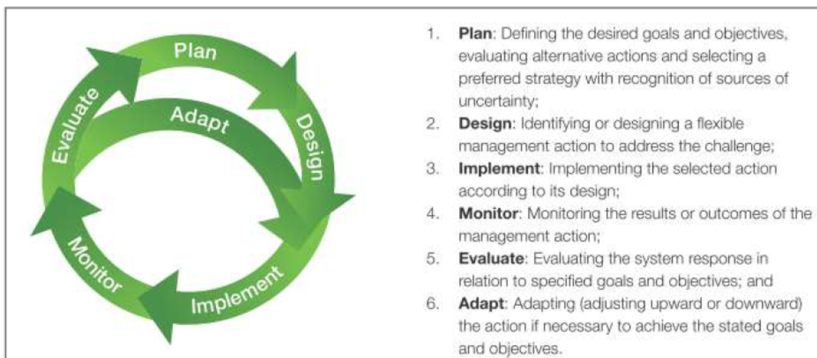
Figuur 21: Principe van Adaptive Management (Bron: CEDA Position Paper integrating adaptive environmental management into dredging projects, Maart 2015)
