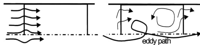
Figure 3.8: Left: Flow pattern over fully submerged groynes. Right: Flow pattern over partially submerged groynes (Czernuszenko and Rowinski, 2005)
