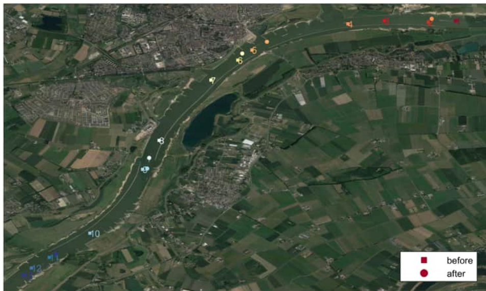
Figure 3.6 Location of the cross-sectional measurements before and after intervention for condition 3. . For each measurement before construction (square marker with number) the matched measurement after construction (circle marker) is given the same color.
