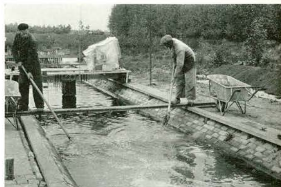
e DUMPING THE MIXTURE OF TRACER AND SAND IN THE DEPOSIT AREA
