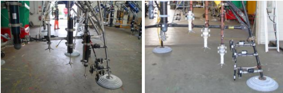
Figure 3.7 Nortek (left) and Sontek (right) ADVs mounted on Frames 4 and 5, respectively.
