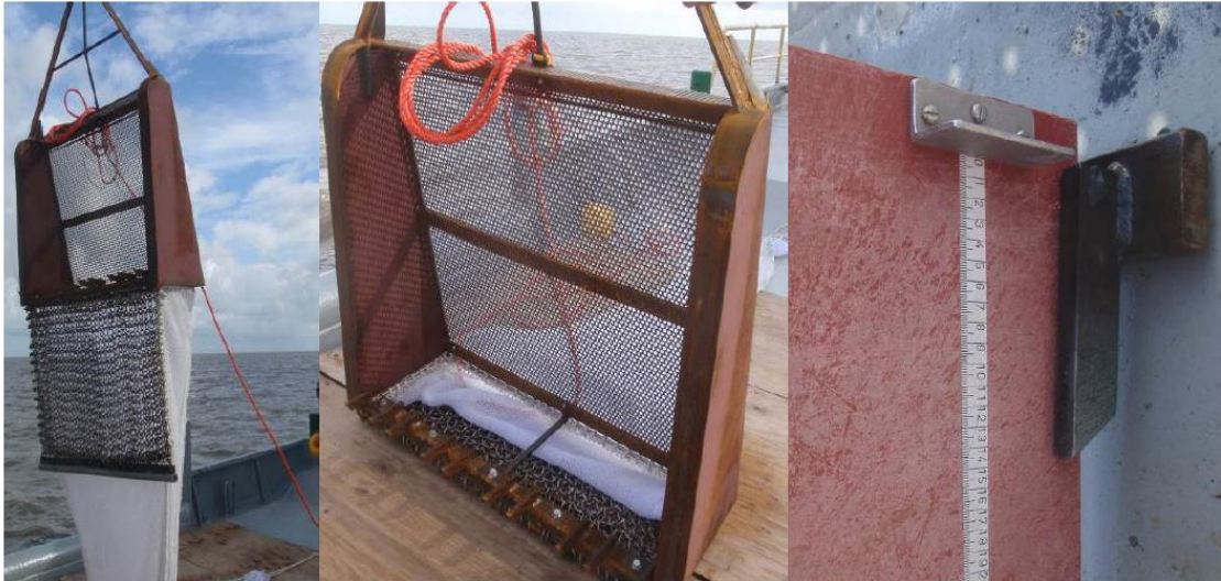
Figure 2.10 Modified 1.24 m shellfish dredge of Rijkswaterstaat.
