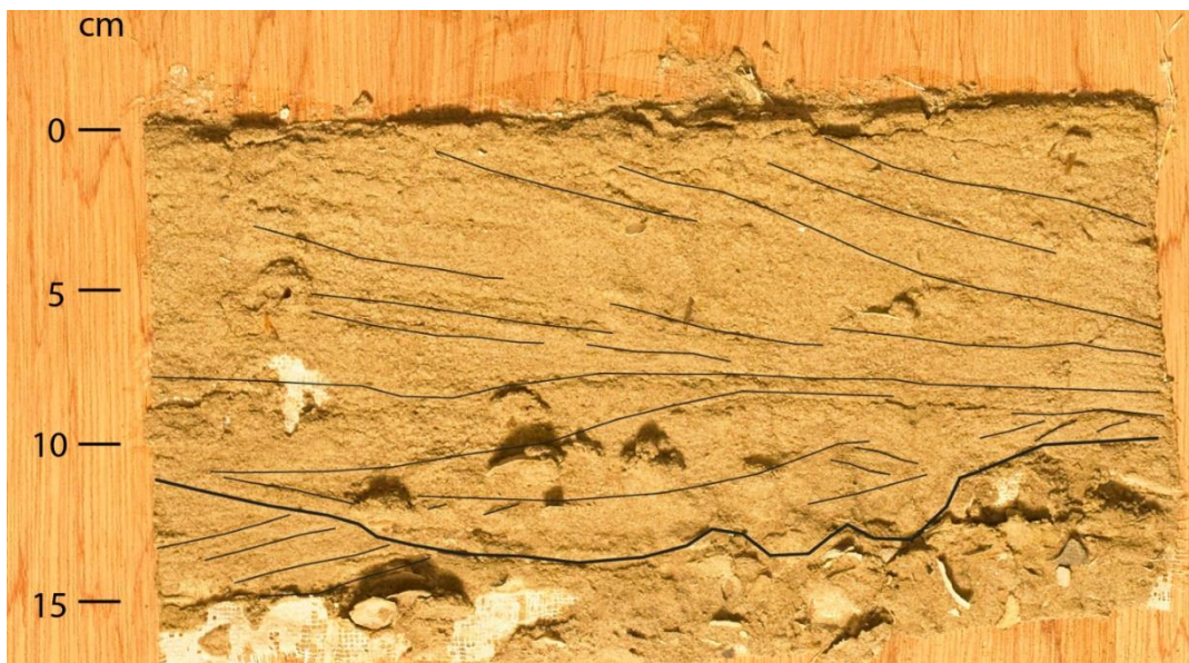
Figure 4.27 Lacquer peel of boxcore AM05, Ameland lower shoreface.
