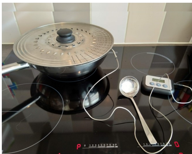
Figure 1. Standard setup for the extraction of non-stick pans with boiling water.
