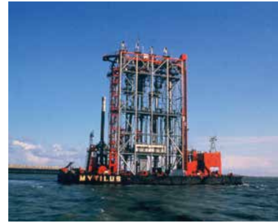
The Mytilus sea-bed compression vessel
